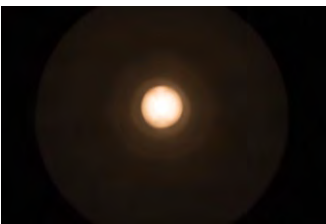
Example high quality flashlight manufacturer A Very small, non-uniformly illuminated surface, strong yellow coloration
